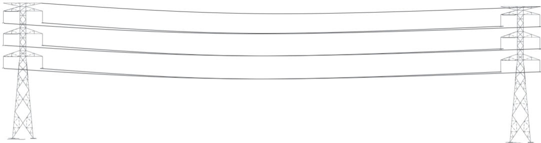
Span generally within 50m to 500m
