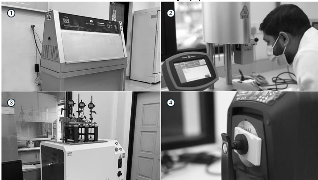
(1): Accelerated weather tester. (2) MFI measurement device. (3) Heat deformation tester. (4) Spectrophotometer.
